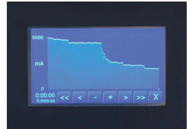
The Parasitic Drain Tester, **PDT Heartbeat 1001**, is an automotive diagnostic tool used to conclusively determine if a vehicle, motorcycle, RV or other 12 volt system has an excessive electrical draw.
